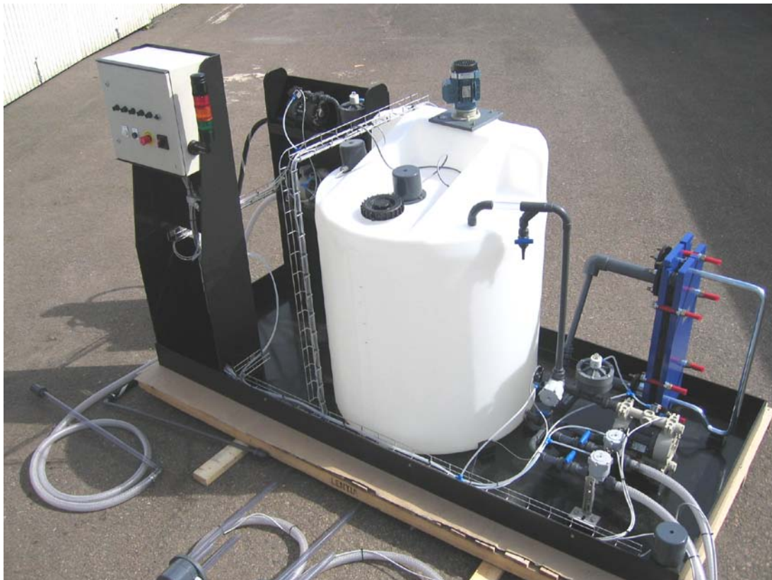
Acid mixing unit
