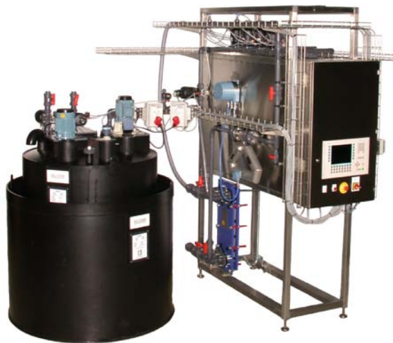
Batch Acid Mixing unit
